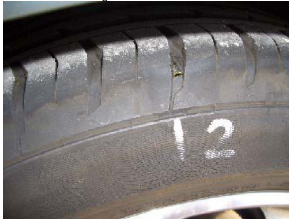
Damage not sealed after 10 km
