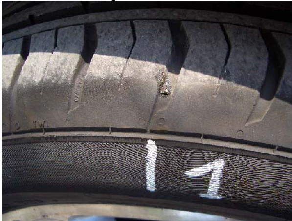
Damage sealed after 10 km
