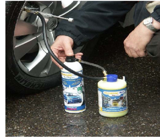
Filling process with AIO aerosol and comfort bottle
