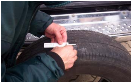
Measuring of the Cut
