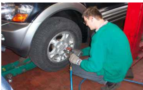
Disassembly After 303 km Test Drive
