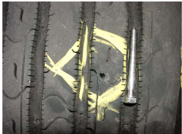
Bolt 8 mm with damage canal
